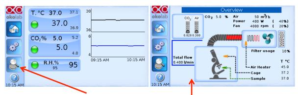
If you press the 'magnifying glass' icon you will see the data from all the sensors in the system depending on the equipment connected.
