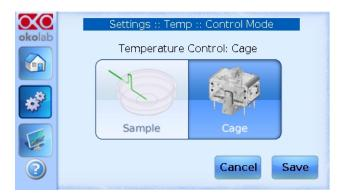
Press 'Cage' if you want to use the white temperature sensor with silver tip as reference. Place the white temperature sensor close to the sample (by the stage, or condenser. Make sure its silver tip is not in contact with metal. Press 'Save'.
